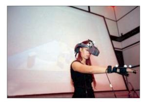
Fig. 1. Head-mounted display and haptic glove
